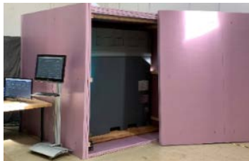
Fig.2.2.1 Thermal chamber at 60°C validating desat conditions
